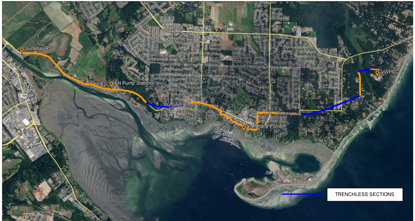
Figure 9 - Options 2 and 3: Trenchless Forcemain Alignment
