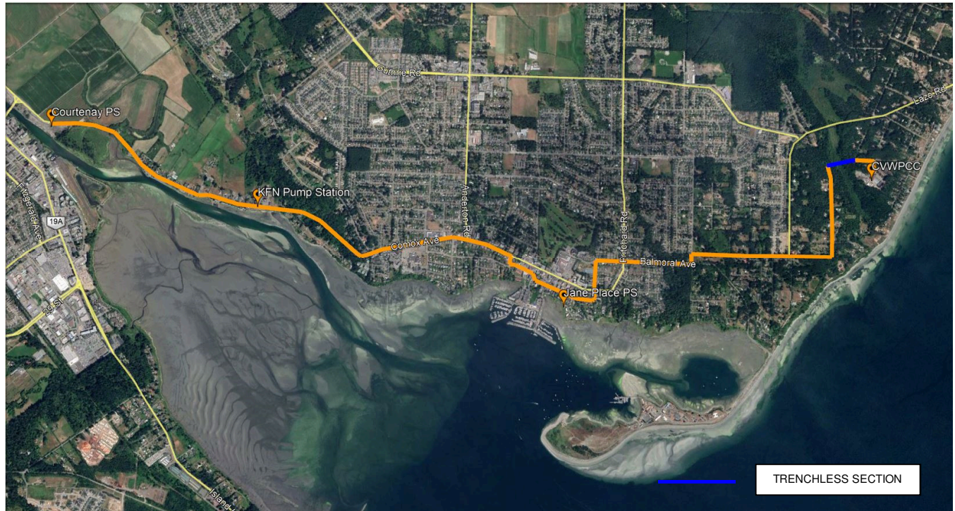
Figure 6 – Option 1: Cut and Cover Forcemain Alignment
