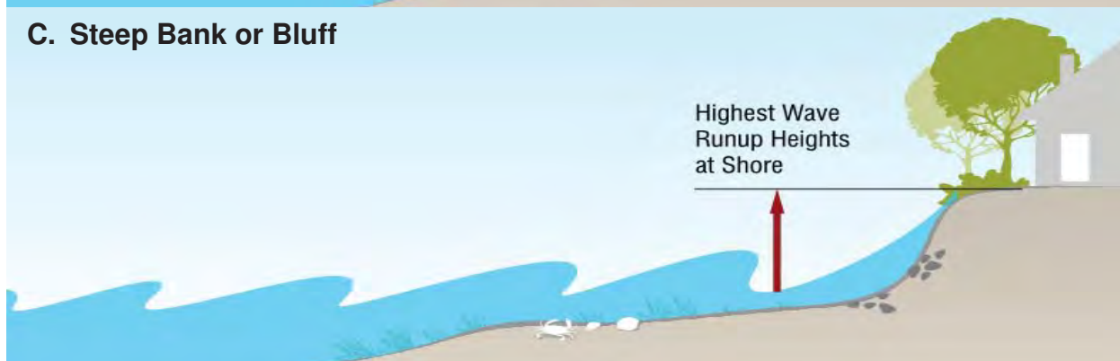
Figure 9: Effect of Different Shoreline Slopes on Wave Runup
