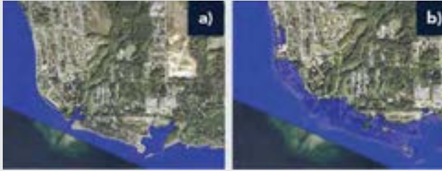
FIGURE 24: Sea-surface height (in purple) during the February 2006 storm surge on the Sunshine Coast Highway (Highway 101) at Davis Bay a) and during a 1 m storm surge with a 1 m of sea-level rise b) . (N. Vadeboncoeur, unpublished data, base image from Google, 2015).
