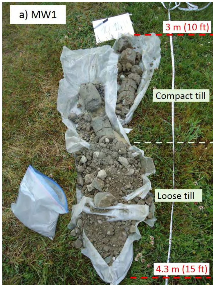
Figure 5. Illustration showing core samples from sonic drill for a) MW1 and b) MW4
